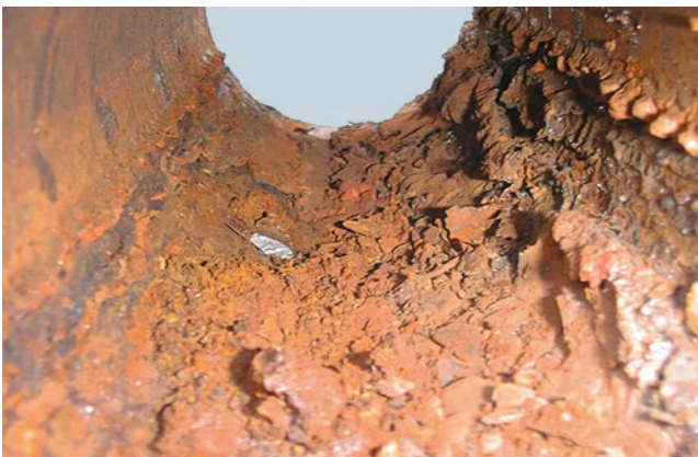
Corrosion on the inside of an untreated pipe
