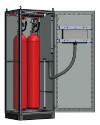
A fire detection control panel integrated in the front door is connected to the detectors, which react to heat or smoke, and activates the extinguishing unit in the event of a fire. The Minimax compact module can be placed in the immediate vicinity of the object to be protected and can quickly be connected with the cable and pipe network using standard connections.
