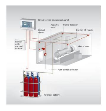
The compressed gas flows into the water cylinders and drives the water into the pipework and onto the nozzles.
