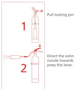
Direct the extinguishing nozzle towards the fire and press the lever.
