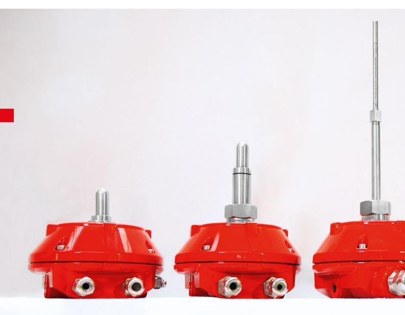
The WMX5000 is designed to detect open fires with rapid heat development, which can occur, for example, with easily combustible plastics or flammable liquids and gases. The heat parameters can be evaluated differentially for early fire detection in addition to the maximum temperature measurement, even in the event of a rapid temperature increase.
