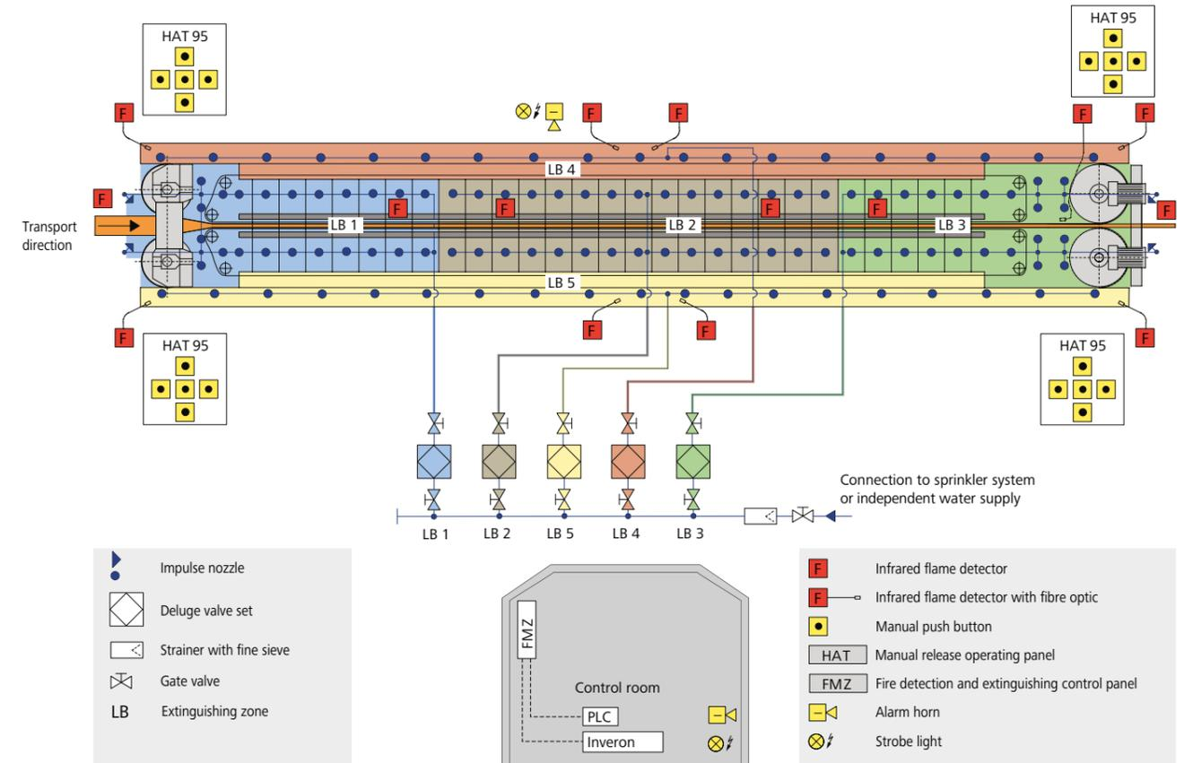
Centralized valve station position (recommended)
