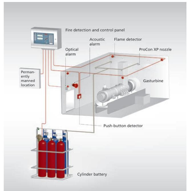
The compressed gas flows into the water cylinders and drives the water into the pipework and onto the nozzles.
