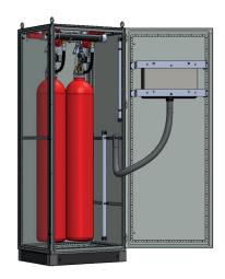
A fire detection control panel integrated in the front door is connected to the detectors, which react to heat or smoke, and activates the extinguishing unit in the event of a fire. The Minimax compact module can be placed in the immediate vicinity of the object to be protected and can quickly be connected with the cable and pipe network using standard connections.
