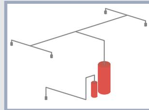
MX 200 fire extinguishing system with asymmetric pipework
