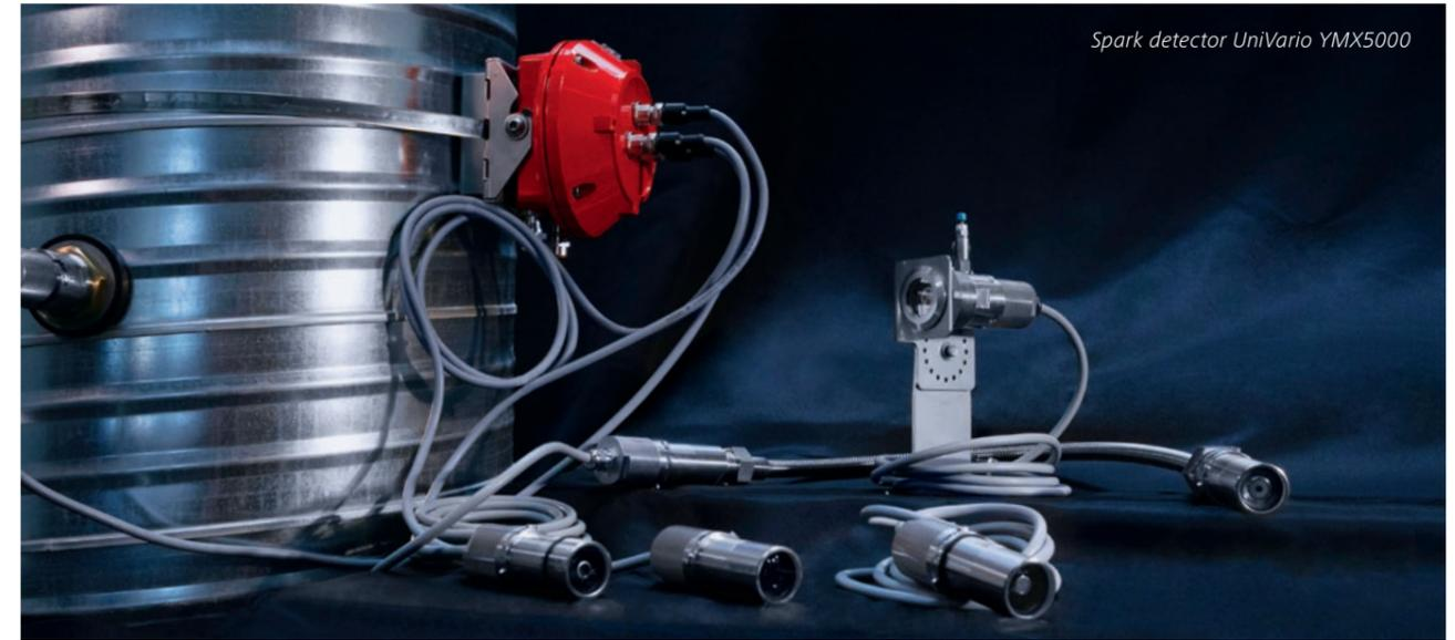
Sparks or glowing embers in the exhaust- and conveyor systems of a wood processing machine must be detected and extinguished quickly. Spark extinguishing systems are the suitable choice for these requirements. Detection is provided by spark detectors of the UniVario YMX5000 series. These detectors have a detection spectrum that is tailored specifically for the detection of sparks or hot parts.
