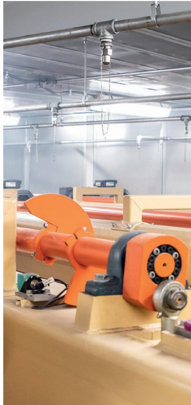
WoodTechProtect combines fire detection, water mist and spark extinguishing technology into a single system. Fire protection for wood processing machines is provided by Minifog ProCon water mist systems, while exhaust
